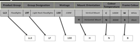
$\textbf{LL3LRF130HNB} \ \textit{LUMEX Light Rack Floodlight 130W Horizontal Mount 4000K Black Frame}$
